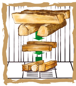
Firing element positioned under the split logs
