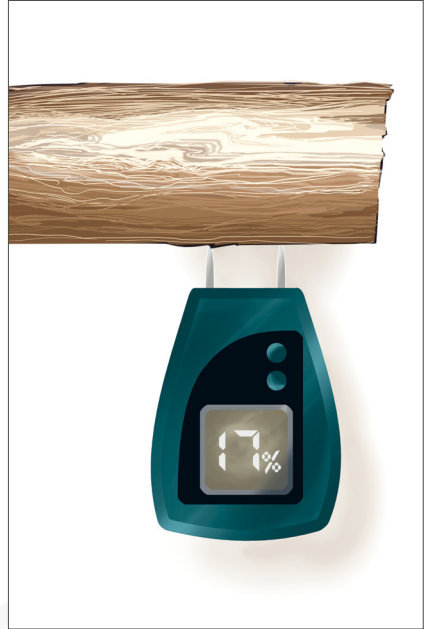
Two electrodes are driven into the wood. The resistance of the current flow shows the residual water content.
