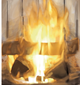
The fire has reached the entire amount of the wood. Now throttle the air supply.
